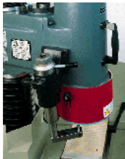
Semi-automatic grinding wheel dresser. All models.
